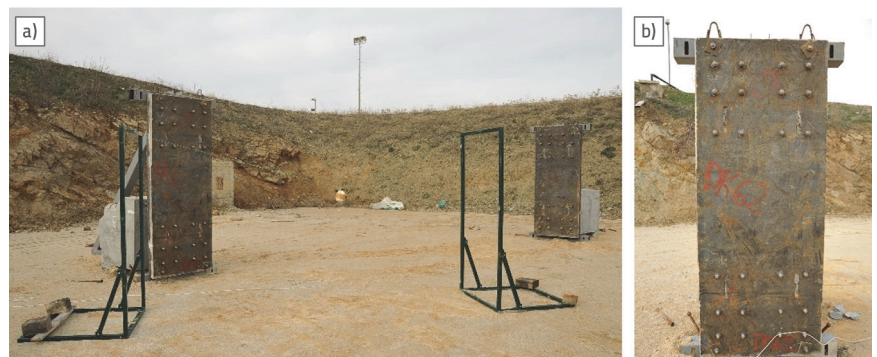
Figure 17. a) C4 blast set 275 cm from the face of the panels; b) Panel face after blast showing minor blast burns but no observable structural damage
